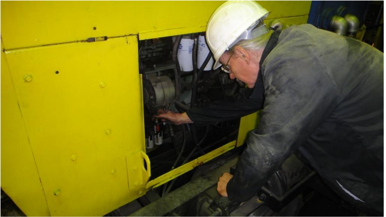
Fred locates the air leak in the tie-shear and begins removing and bypassing the air-dryer
